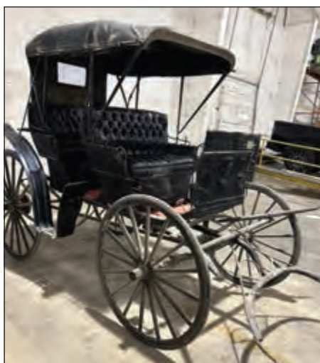
- Black, two-seated, horse drawn carriage in good condition. Has a top and a single tongue with double tree for a team. Also has brakes. Nameplate on the back but we cannot read it. Has been kept in a shed.
