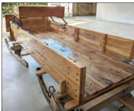
- Bobsled with complete original wood and metal of the original unit. Bobsled box is a handmade reconstruction made from ash lumber, milled from trees on the seller's property.
